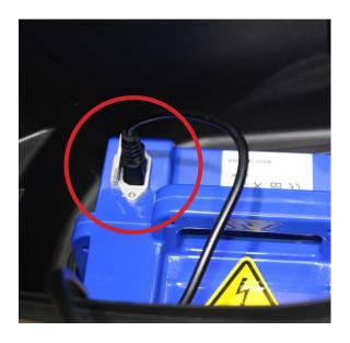
7. Connect the IEC C13 connector from the charger to the battery, we need to lift the top that cover the connection in the battery.
