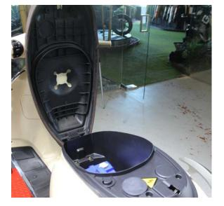
3. Lift up the seat to Access to the battery connections.
