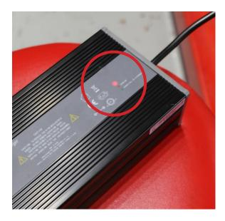
8. Wait a few seconds and check out that the LED indicator of the charger is on with RED light.
