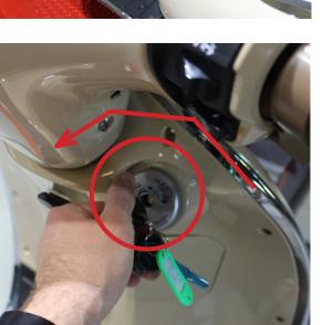
1. To access to the battery, it will be necessary put the key inside the start lock.
